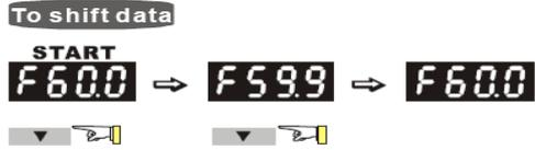
**Setting direction** (When operation source is digital keypad)
